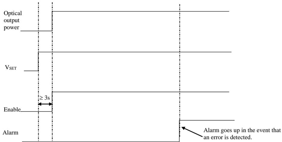
Figure 3 Startup and operational timing of the module
