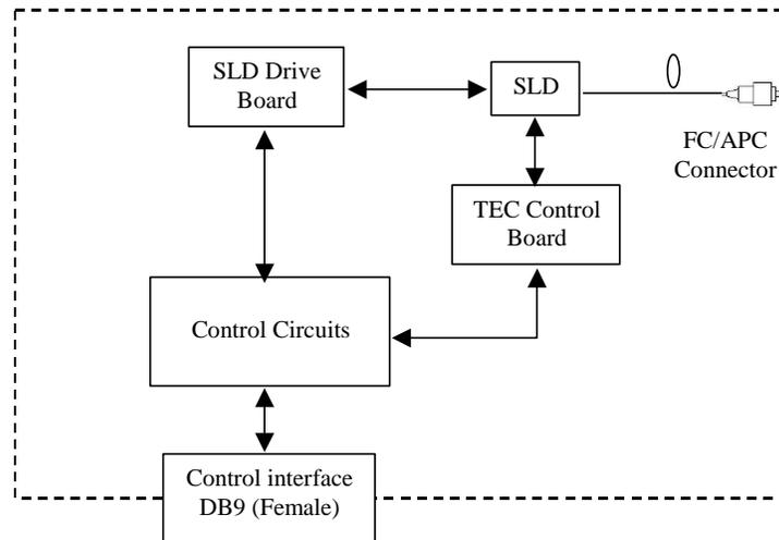
Figure 1 Configuration of IPSDS1304-xxxx SLD light source module
